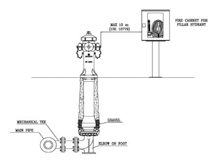
TECHNICAL CHARACTERISTIC: Underground part must be at list 300 mm deep from ground level to automatic drainage
