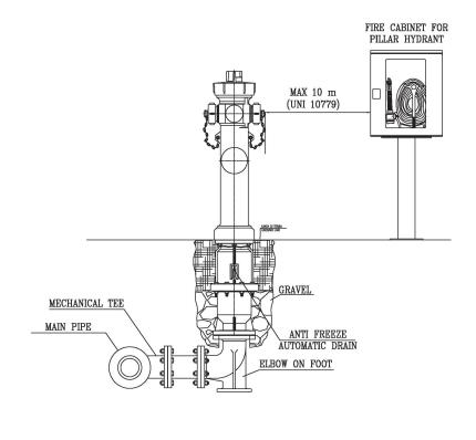
TECHNICAL CHARACTERISTIC: Underground part must be at list 300 mm deep from ground level to automatic drainage
