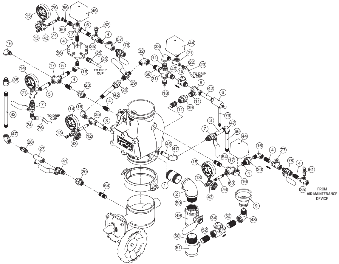
FIGURE 12: 6" RCW SINGLE INTERLOCK PREACTION DRY PILOT ACTUATION TRIM ARRANGEMENT
